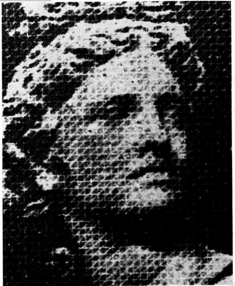
Fig. 13. Enlarged detail (10x) of Talbot photogravure screen (ca. 1852) incorporating a double "working-type" screen.
