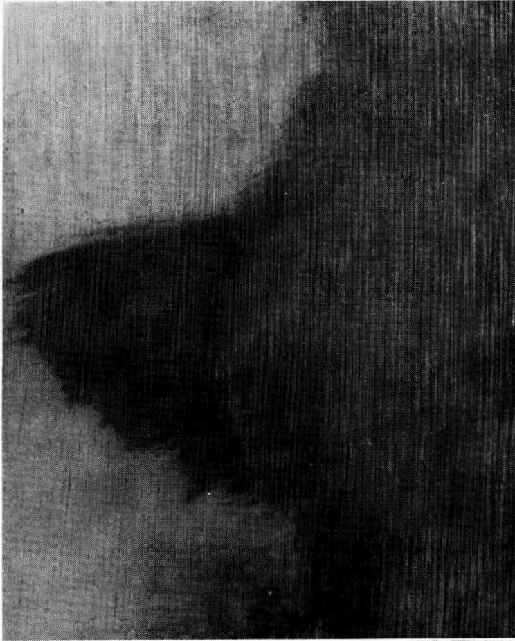
Fig. 8. Enlarged detail (10x) of a Talbot screen, a transparent, flexible sheet of cartilaginous-like material containing nearly parallel, short lines scored into both sides of sheet. Ink has been rubbed into a small area to illustrate appearance of opaque lines.
