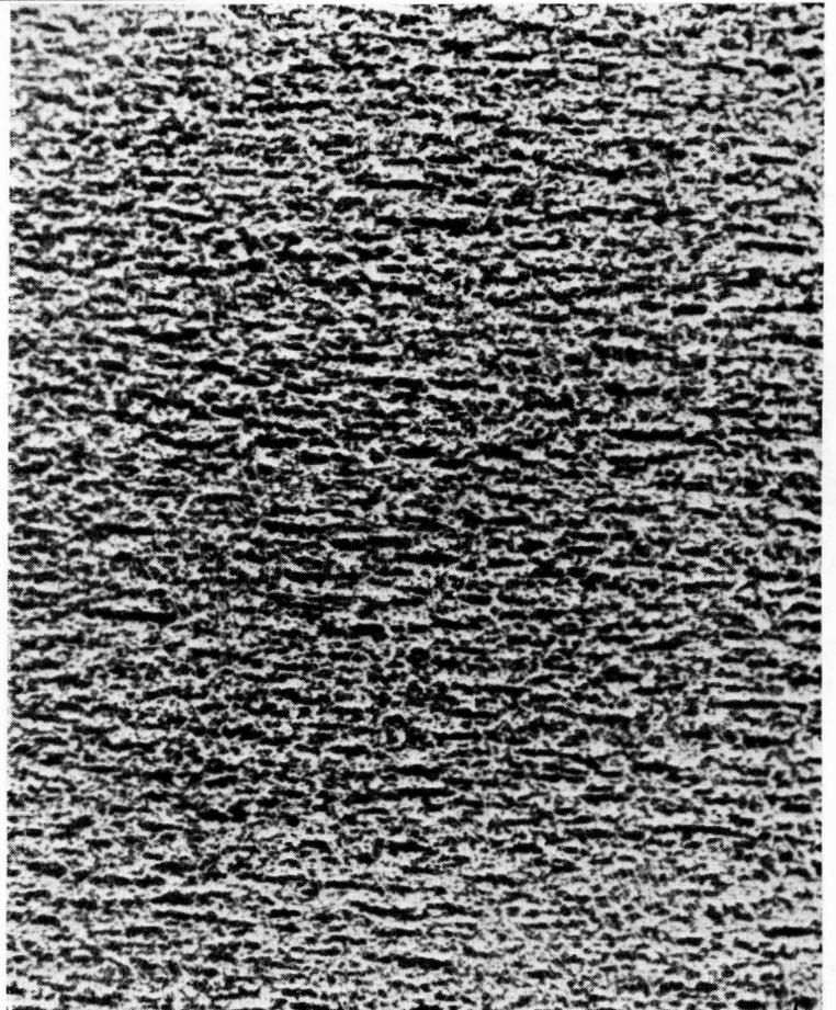
Fig. 9. Enlarged detail (10x) of a Talbot screen on paper: lithographic paper print (probably from crayon drawing on stone), waxed for improved translucency.
