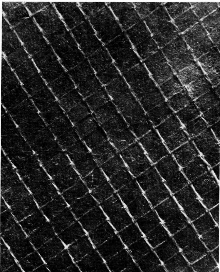
*Fig. 6. Enlarged detail (12x) of Talbot's yellow gauze screen embedded in a transparent flexible film to hold fibres firmly in place. Areas between fibres are actually transparent but here they appear dark because reflected surface light was used to help emphasize screen fibre details.*
