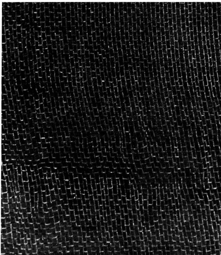
Fig. 5 Enlarged detail (Bx) of yellow gauze screen used by Talbot. Note similarity of mesh pattern with that shown in dig. 3. Dark background was used to help emphasize screen fibre details.
