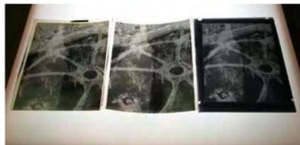
*Left:* two 5x4 nitrate negatives and a copy negative on glass. *Right:* four silver gelatin DOP prints of varying dimensions, a 17x14 platinum print and a 17x14 negative on Cristoid film.
