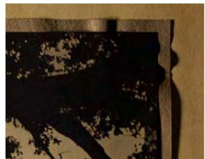
The adhesive used to tip prints to secondary supports has progressively lost its adhesion properties, so that photographs have detached from their mounts. In addition, the adhesive discoloration has affected some works in their aesthetics.
