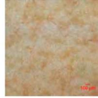
It is unclear if these are a manifestation of deterioration of the paper support due to residual iron salts in the platinum process, or if they are instead related to the gum layers.
